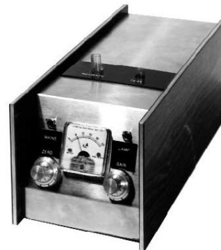
Figure 5: The first aggregometer made in the workshop at the Royal College of Surgeons in 1961. Born (1962b).
